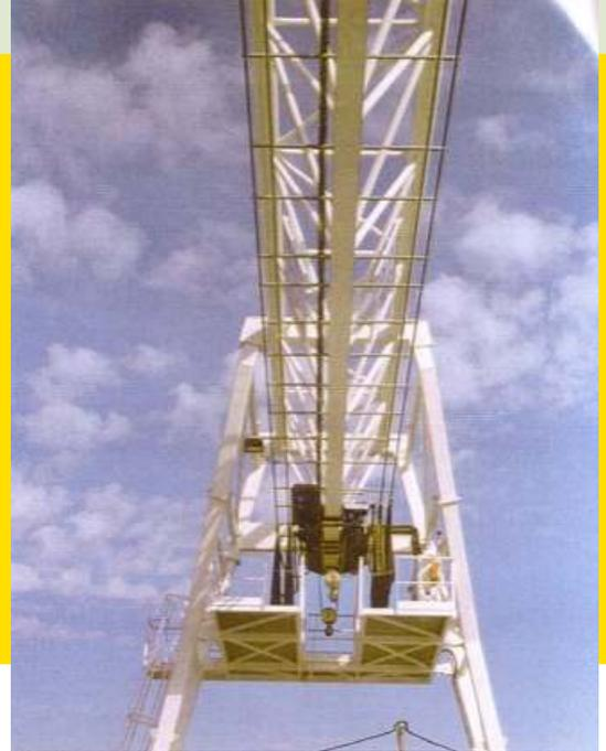
Portal Cranes with a lattice structure, are designed to reduce the maximum surface area against wind resistance, optimising its power for the long travel movement.
