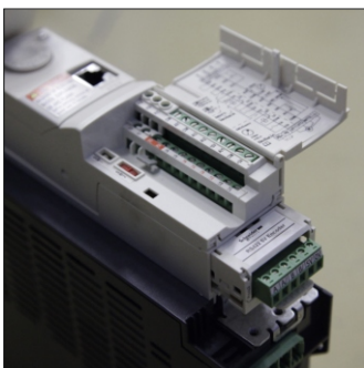
11 Hoist Frequency inverter
